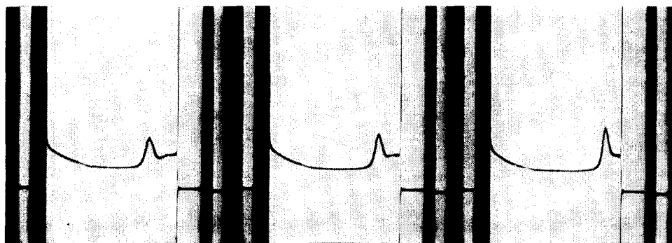
Fig. 5. Sedimentation of purified lactase. Conditions: 3 mg protein/ml; 0.1 M NaCl; 59 780 rev./min; rotor AnD. Pictures shown here: after 16, 24, 32 min.
